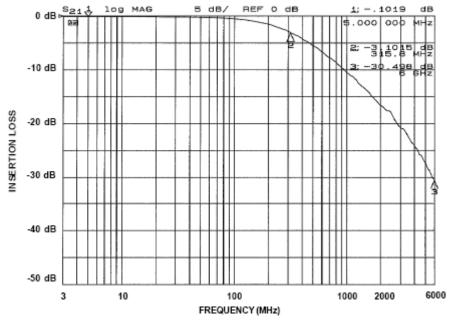
Figure 4. Insertion Loss vs. Frequency, Filter 4 (Pins 4 and 5)
