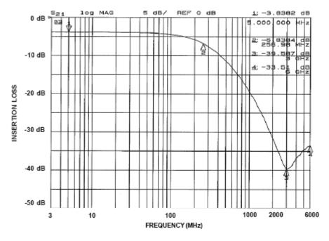
Figure 2. Insertion Loss vs. Frequency, Filter 2 (Pins 2 and 7)
