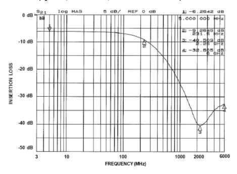
Figure 3. Insertion Loss vs. Frequency, Filter 3 (Pins 3 and 6)
