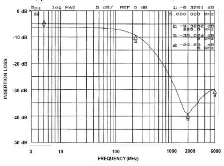
Figure 1. Insertion Loss vs. Frequency, Filter 1 (Pins 1 and 8)
