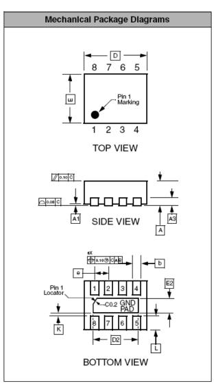
Dimensions for 8-Lead, 0.4mm pitch UDFN Package
